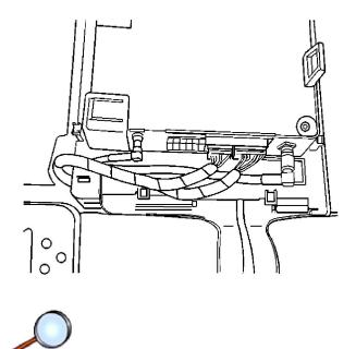
2. Install the module to the upper bracket ensuring the retaining tab is fully seated.
